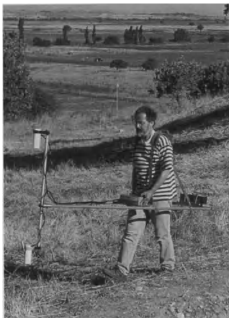
Fig. 10. Magnetic prospecting with a cesium magnetometer (Geometrics, two mobile sensors, third stationary sensor seen in background) west of the citadel. (N. Blindow 1999)
