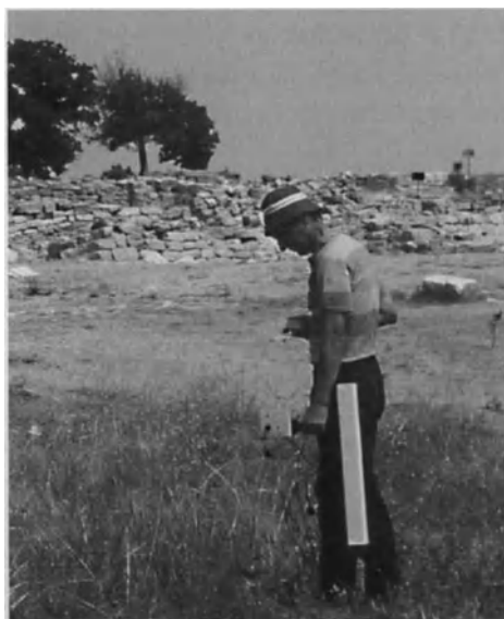
Fig. 4. Magnetic prospecting near the agora of Troia with the fluxgate gradiometer. (H.G. Jansen 1988)
